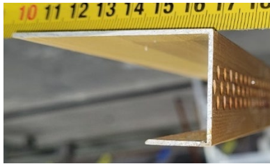
Photo No. 10 Starter track profile
