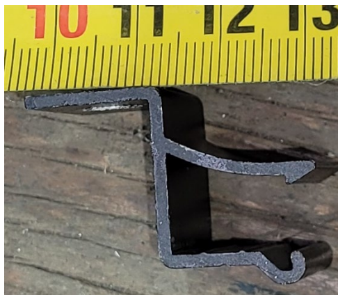
Photo No. 8 Installation clip profile
