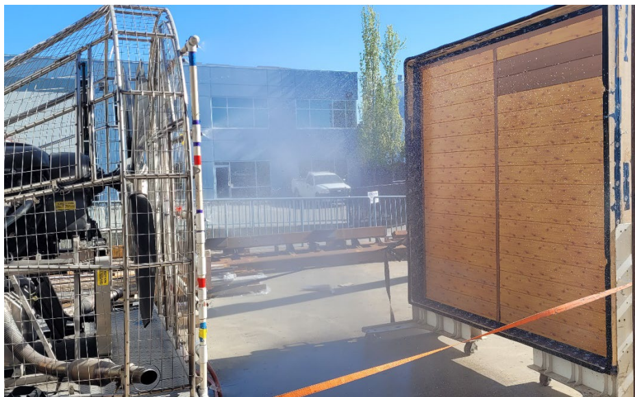
Photo No. 2 – Aluminum Siding - Rain Screen System – AAMA 501.1 test setup
