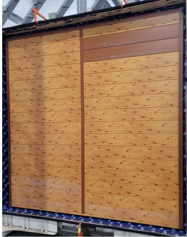
Photo No. 1 – Aluminum Siding - Rain Screen System
