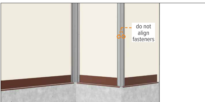
Figure 17.2 Installation Guide for QuickPanel Systems®
