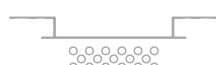
Perforated Soffit 5/16" Trim Net Free Air Space 7.7 in 2 /lin ft 163.3 cm 2 /lin m
