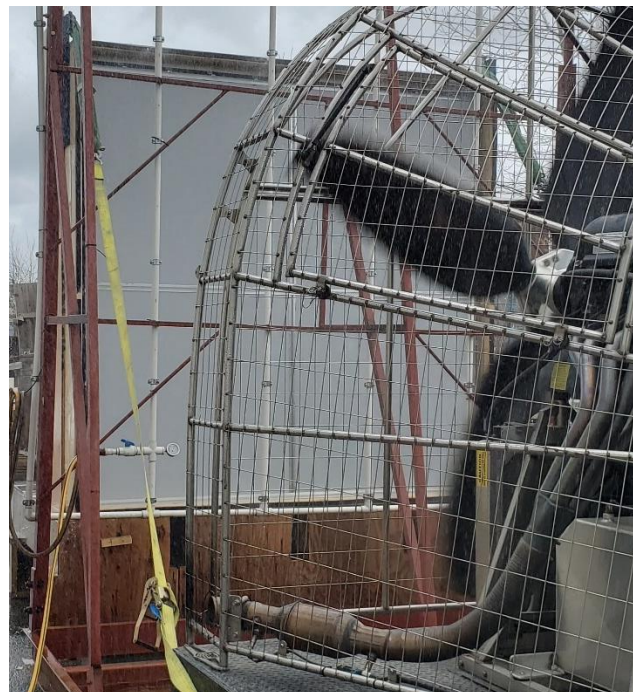
Photo No. 3 AAMA 501.1 - Dynamic water test setup
