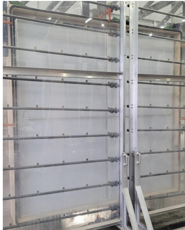
Photo No. 2 ASTM E331 – Static water test setup
