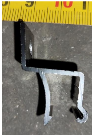
Photo No. 7 Installation clip profile
